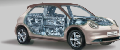
65% High Strength Steel Throughout Vehicle Body
